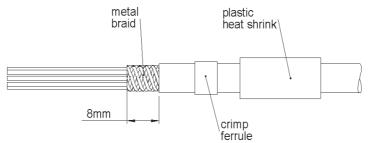
Put wires through and shape cable metal braid around the anchor ferrule.
