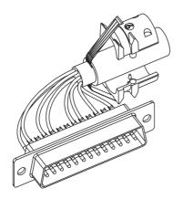
Turn the pigtail cable shield back over the strain relief. If not using any strain relief from the supplied set, use the same procedure around the outer cable jacket.
