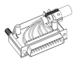
Complete the assembly by putting the top half over the assembly and tighten with accompanied assembly screws. Maximum mounting torque is 100 - 120 Ncm.
