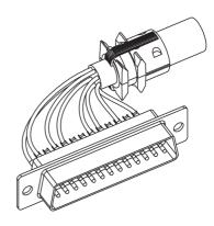
Place the assembled connector and cable into the bottom back shell half.
