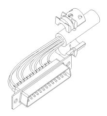
Mount connector and cable into the back shell.
