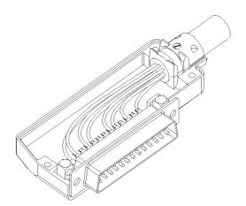
Assemble bottom half and top half with the three assembly screws. Maximum mounting torque is 100 - 120 Ncm.
