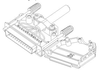
Close the hinged back shell and assembly is completed.
