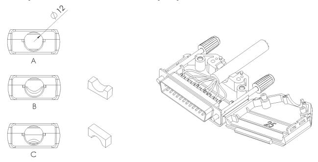
Place the mounted cable and connector inside the back shell. Mount the cable clamp and assembly screws. Maximum mounting torque is 100 Ncm.
