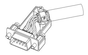
Mount the top back shell half with the accompanied assembly screw. Maximum mounting torque is 80 - 100 Ncm. Assembly is now completed.
