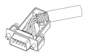
Fasten the cable clamp with the two cable clamp screws enclosed the kit.
