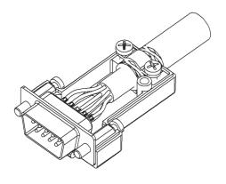
Mount the top back shell half with the accompanied assembly screw. Maximum mounting torque is 80 - 100 Ncm. Assembly is now completed.
