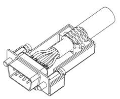
Fasten the cable clamp with the two cable clamp screws enclosed the kit.
